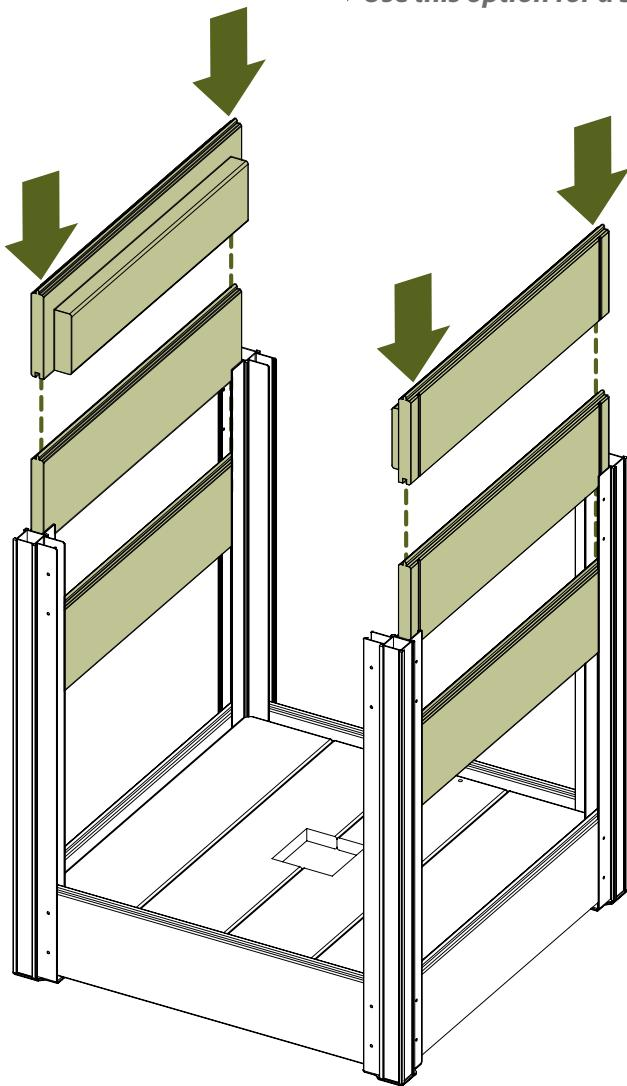
! Top support boards (C) should be on the opposite 2 sides as the bottom support boards.
